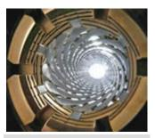
Inoex's vacuum calibration tank uses lattice-like interwoven steel straps to change pipe length and diameter over a 4:1 range. <u>Rollepaal</u> added flaw-detection software to its static ultrasonic array for pipe thickness testing. The static array has 28 non-contact ultrasonic scanners for pipe under 8 in. diam.
