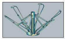
Hungarian stretch-film processor DR-Pack offers its unusual IBC apparatus, which blows air tangentially onto the bubble. DR-Pack also developed an adjustable IBC system, which opens like an umbrella with air coming out the spokes tangentially onto the inside of the bubble. The air ring outside the bubble blows tangentially in the opposite direction, keeping the bubble more stable than a conventional air ring and IBC, DR-Pack says.
