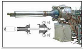
Frankische Rohrwerke's quick-change preassembled pipe die takes 90 min to change and start up, vs. 10 hr for a conventional die.
